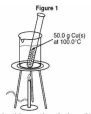
In a laboratory investigation, a 50.0-gram sample of copper is at 100.0°C in a boiling water bath.
