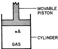
As the piston moves toward point A at constant temperature, which relationship involving pressure (P) and volume (V) is correct?
