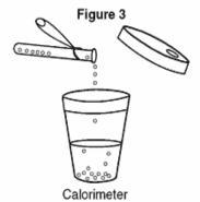
The hot copper is poured into the cup of water, and the cup is quickly covered with the lid.
