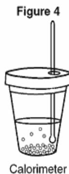
A thermometer is inserted through the lid. The copper and water are gently stirred in the cup. The temperature is checked periodically. The highest temperature noted is 26.3°C.
